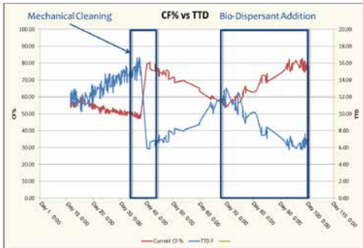
Figure 4 - The comparative effects of the mechanical cleaning and bio-dispersant application are shown in this graph from the plant's DCS.
